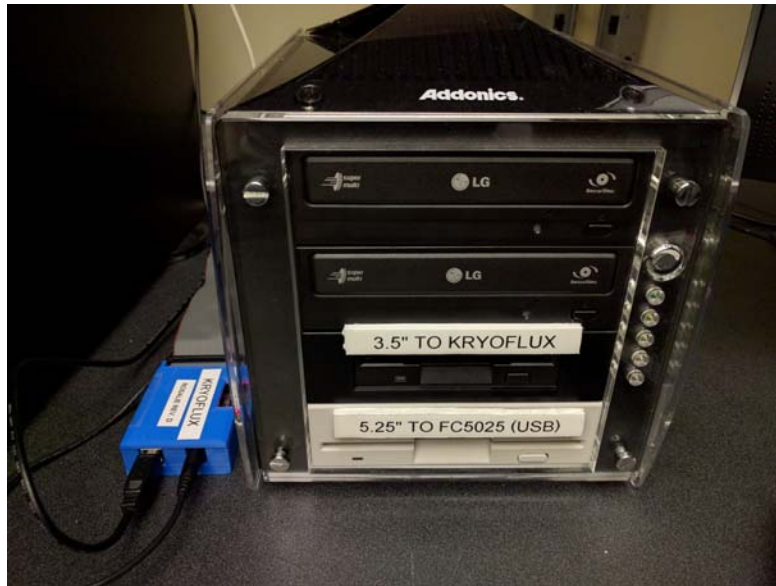
Kryoflux Running on a "Mini JukeBox"*
