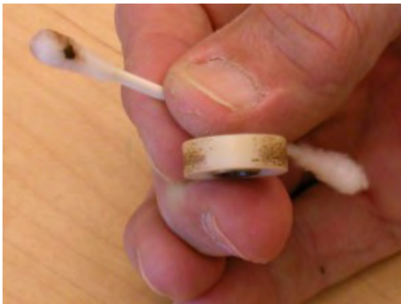
Flakes of iron oxide from a tape suffering from sticky-shed syndrome. Photo courtesy of Nicholas Wojcik.
