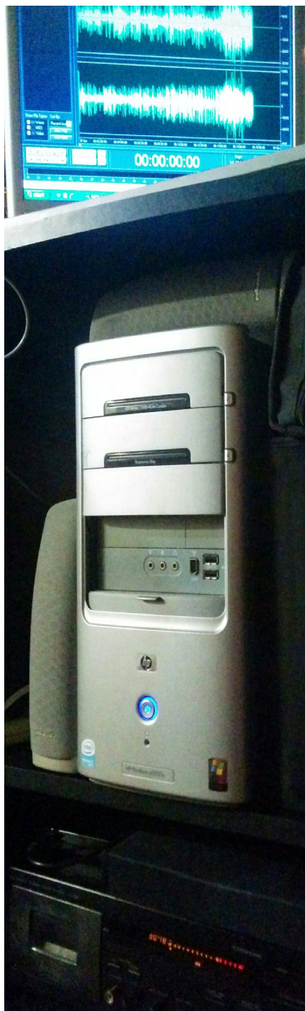
Author's home analog-to-digital conversion workstation, using Yamaha cassette deck output via RCA cable to 1/8" inch jack into HP desktop computer running Cool Edit Pro version 2.1.1. Photo courtesy of Brett Dion.
