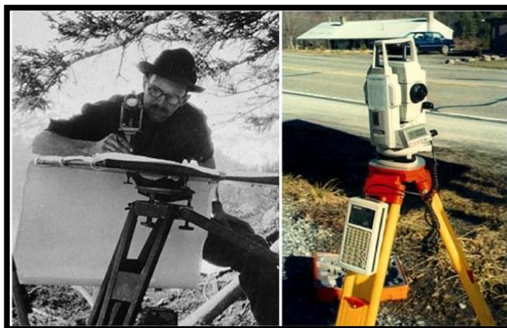
Figure 1. Old vs. new ways to collect archaeological data — an alidade and a total station. 2
