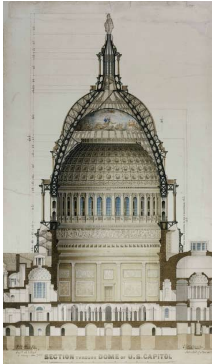
Section Through Dome of U.S. Capitol by Thomas U. Walter. (Architect of The Capitol)
